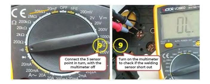
Check carefully for cold solder faulty joints or short from solder.
