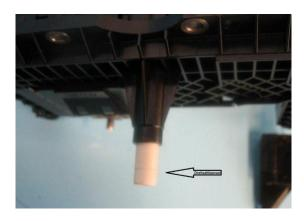
**Example:** Speed sensor and bracket broken off
